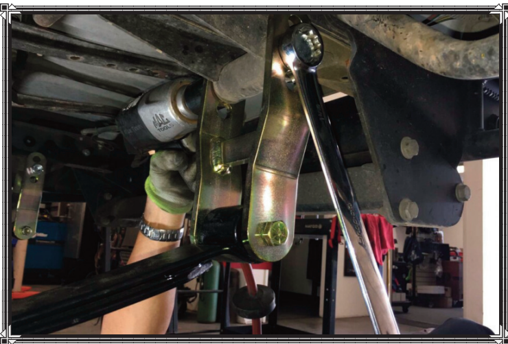
Before lowering the vehicle back on the ground, the rear shackles were installed snugly on both ends. Once the vehicle was on the ground and settled in position, we tightened the provided locking nuts (being careful not to overtighten).
