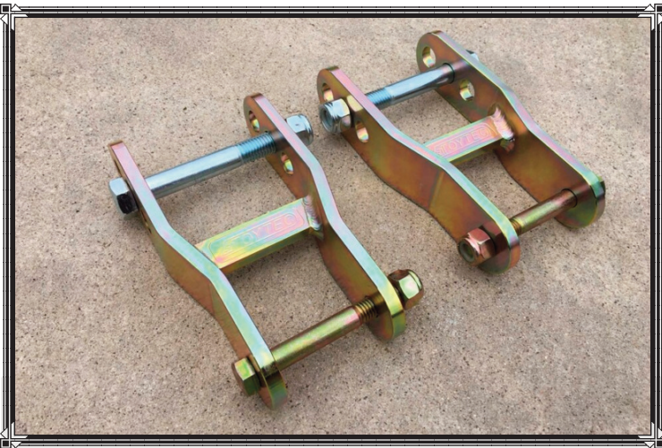
These adjustable-lift-height SKL2 shackles from Toytec were a perfect solution when going back to a factory 14mm spring bushing while still attaining 1, 1.5, or 2 inches of additional lift.
