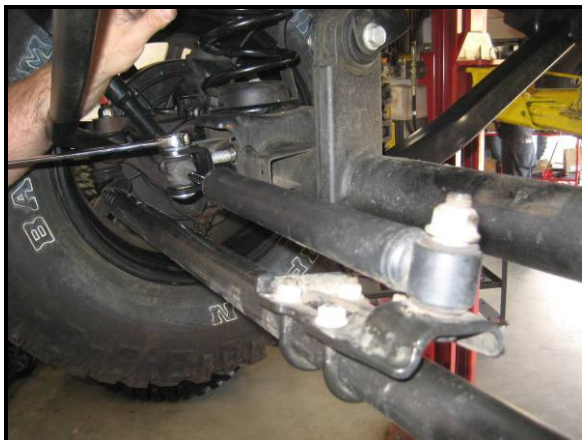
Photo 23 Loosen factory stabilizer bracket on tie rod and roll to top of tie rod. With wheels straight ahead, and stabilizer extended to half way mark, tighten stabilizer bracket and bolt at new bracket. Cycle steering and verify clearances.
