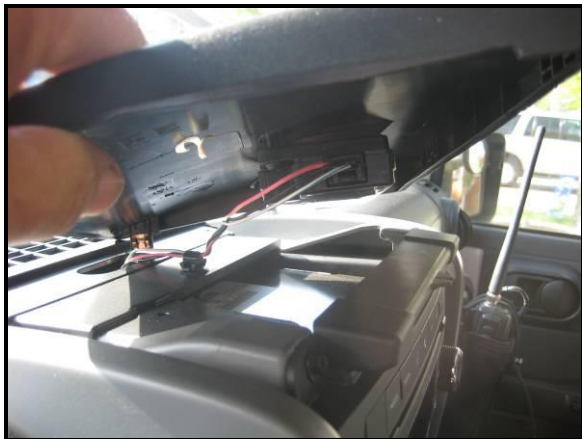
Lift the factory panel from the dash. Be careful not to damage the compass module wires.
